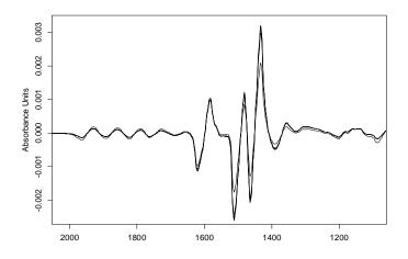
1<sup>st</sup> derivative of 5 polystyrene film spectra showing excellent wavelength precision.
