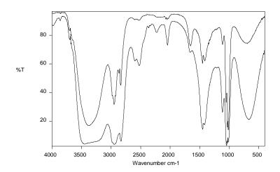
Methanol with different sample thickness
