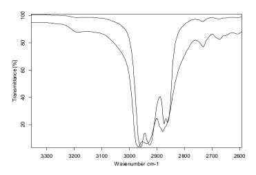
C-H stretching region showing effect of specular reflection from sample surface
