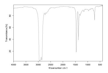
Lubricating oil measured at 4 cm<sup>-1</sup> resolution, 5 second measurement. Spectrometer: Bruker Vector 22
