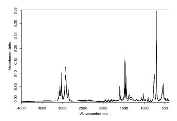
Polystyrene film cast from xylene: 5 replicate sample measurements 4 cm<sup>-1</sup> resolution, 5 second measurement on DPT Sampler
